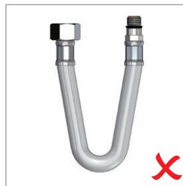
*The hoses must maintain a straight section at the connections equal to 4 times the external diameter of the hose (DN6 = Ø 10 mm → straight section 40 mm).*
