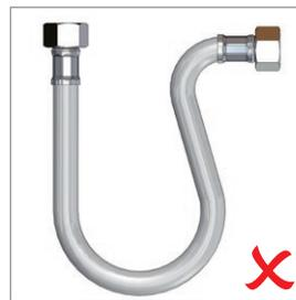
*Design the system using hoses of adequate length and fittings to minimise hose twists and tensions (always check the product datasheets).*
