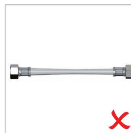
*Do not install flexible hoses under twisting or tension conditions.*
