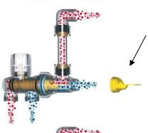
If the flow direction is not observed with valves M 85 and M 86, it is necessary to correct it by turning the baffle inside the conveyor body . riprendere il giusto verso del flusso. Use the baffle as shown in the picture to let the flow enter through the connection as displayed by the arrow.
