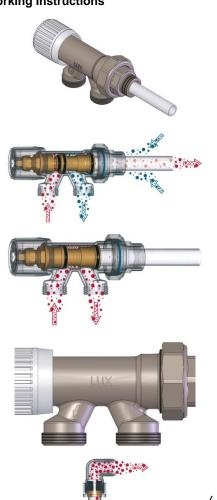
The M 87 valve has a fixed bypass, in full open position 50% of the ring flow rate enters the heating body.
