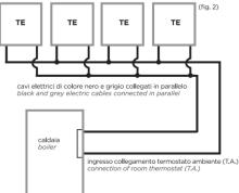
Connection of thermoelectric heads with limit switch contact and boiler with "room thermostat".
