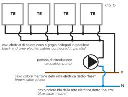
Connection of thermoelectric heads with limit switch contact and circulation pump for heating systems.
