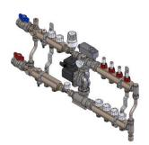
The version with KA1191 allows for control and balancing of the incoming water, but not using a way of the manifold. Moreover, by connecting another manifold to the KA1191 it is possible to control the distribution both for the high temperature and the radiant panels circuit with a single system. This type of system can supply a max thermal power of 14 kW with a  $\Delta t$  of 10 °C and a temperature of  $\geq$  70°C on the primary circuit.
