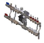
• The version with KA1191 allows for control and balancing of the incoming water, but not using a way of the manifold. Moreover, by connecting another manifold to the KA1191 it is possible to control the distribution both for the high temperature and the radiant panels circuit with a single system. This type of system can supply a max thermal power of 14 kW with a Δt of 10 °C and a temperature of ≥ 70°C on the primary circuit.
