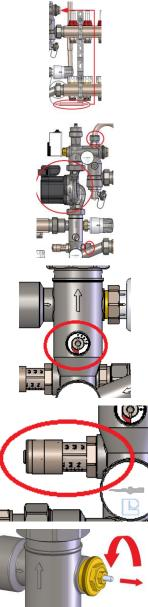
The circulation of water through the secondary circuit radiant panels is activated by the pump featured in the GM 1192, while the thermostatic head mounted on the adjustment valve keeps the temperature of the water to be sent to the radiant panels constant by acting on the quantity of hot water which is integrated into the secondary circuit.
