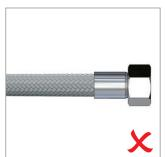
The hoses must maintain a straight section at the connections equal to 4 times the external diameter of the hose (DN6 =  $\emptyset$  10 mm → straight section 40 mm). The bending radius must not be less than 4 times the external diameter of the hose (DN6 =  $\emptyset$  10 mm → bending radius 40 mm).
