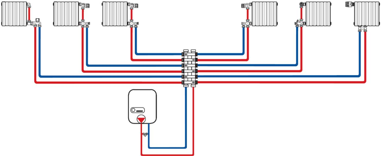
Plastic, copper and multilayer pipes can be connected to all the abovementioned manifolds by using the appropriate TP and TR compression fittings.
