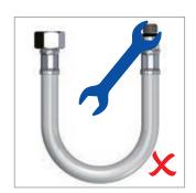
Do not use any tools on the ferrules. A force applied to this ferrule often causes it to become damaged with consequent breakage of the hose.
