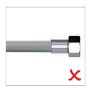
The hoses must maintain a straight section at the connections equal to 4 times the external diameter of the hose (DN6 =  $\emptyset$  10 mm  $\rightarrow$  straight section 40 mm). The bending radius must not be less than 4 times the external diameter of the hose (DN6 =  $\emptyset$  10 mm  $\rightarrow$  bending radius 40 mm).
