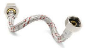
Pipe for connection of household appliances in diameters DN8, DN10 and DN13. The external stainless steel braid guarantees durability and resistance to external agents, maintaining a discrete flexibility as well as a high resistance to pressure and temperature, ideal for hot water. Available with stainless steel braid and socket and brass fittings.
