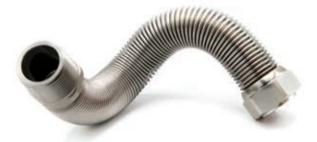
For the connection between the water network and the wall boilers. Extendable metal hose with stainless steel bellows available in different sizes to meet the needs of the installer and the manufacturers of wall-hung boilers.
