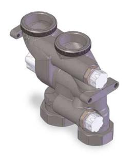
Mixing valve DN 25. This valve can be combined with the thermostatic head TT 3051 for fixed point systems, or to an actuator with a M30x1,5 thread, closing point 11,5mm and stroke  $\geq$  3mm.
