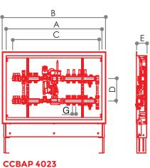
Distribution system for low temperature heating + 3 connections for high temperature (W24x19).
