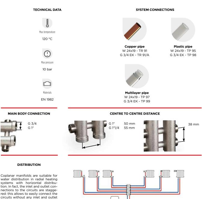
nifold bodies are produced by casting from EN 1982 brass with limited lead content.
