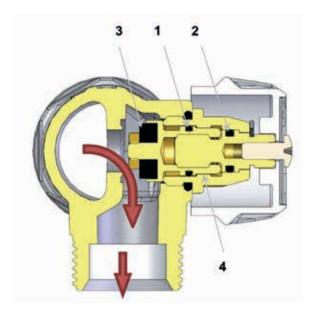
The modular manifold with front shut-off valves must be installed with the inlet water flow as shown in the image on the side.
