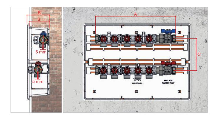
The chart below shows the overall dimensions for the combination of two modular manifolds and a full-flow ball valve.
