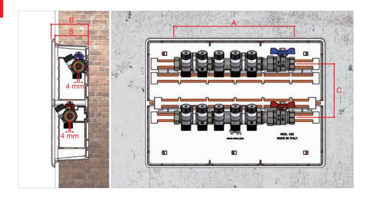
The chart below shows the overall dimensions for the combination of two simple modular manifolds and a full-flow ball valve.
