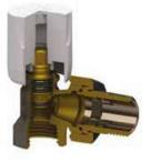
When in closed position, the tightness is granted by an o-ring and a conical metal collar. The valves are nickel plated. Valves and lockshields must be opened with a differential pressure lower than 1 bar.
