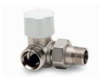
The coaxial valves have a headwork hat allows pre-regulation thanks to a shaped acetal ring. The thermostatic head allows the replacement of one of the sealing o-rings on the control rod without having to empty the system. The valves are produced with a nickel-plated finish.
