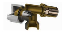
Manual M valves feature a fixed stem, whose tightness is ensured by an o-ring and a flat PTFE gasket which may be adjusted through a brass stuffing nut. When in closed position, the tightness is granted by an o-ring and a conical metal collar. The screw of thermostatic M valves allows to
