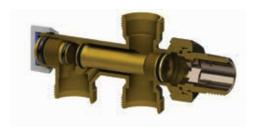
The tightness of distributors towards the outside is ensured by an o-ring and a flat gasket inside the plug. When in closed position, the tightness is granted by an o-ring. The distributors are nickel plated. All distributors allow for flow adjustment by limiting the lift of the obturator.
