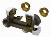
The tightness of distributors is ensured by an o-ring and a flat gasket inside the plug. When in closed position, the tightness is granted by an o-ring and a conical metal collar.
