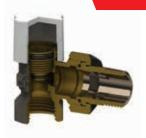
The screw of ThermoTekna valves allows to preset the flow thanks to a shaped acetal ring. The thermostatic screw enables to replace one of the o-rings on the control stem without draining the system. The valves - where clearly indicated - are approved according to UNI EN 215.
