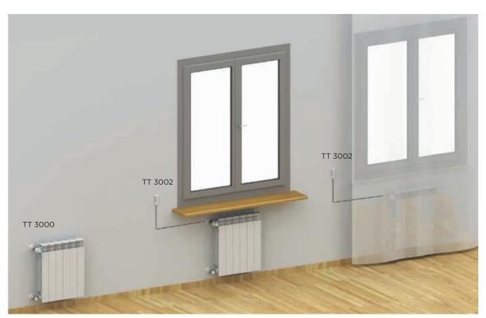
**TT3000** thermostatic heads can be applied to all heating bodies unless in presence of barriers such as shelves, curtains or furniture, which may accumulate heat and therefore alter the measurement of room temperature. In this case, it is recommended to use **TT3002** thermostatic heads with remote sensor.
