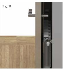
Should the heating body be installed as in fig. 1, a number of issues may arise. The door could not be opened completely and, unless provided with a doorstop, it could hit and damage the head.
