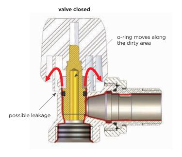
The benefit of the rod made in two pieces are many and occur both with the valve open and with the valve closed. The fixed rod, with double o-ring, guarantees the seal and prevents impurities from settling in the seat where these gaskets work, avoiding the decrease in their effectiveness.
